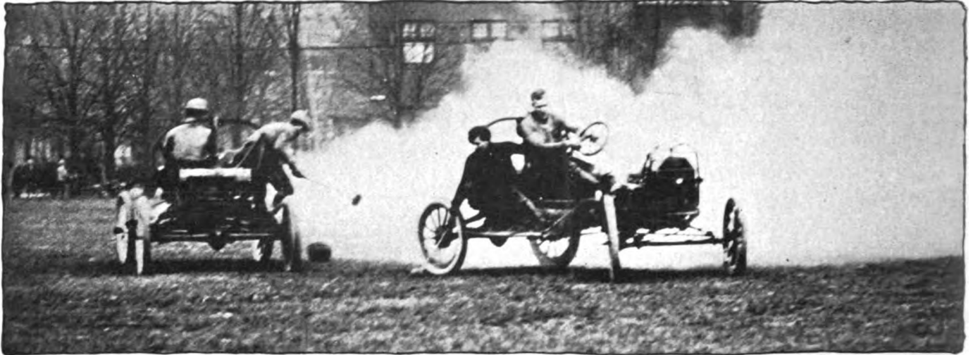
Trying out the new game of automobile polo in Detroit, Mich. The circular bridge steel support on the cars is for the protection of the drivers in the event of the machines turning turtle as they frequently do in this pastime
